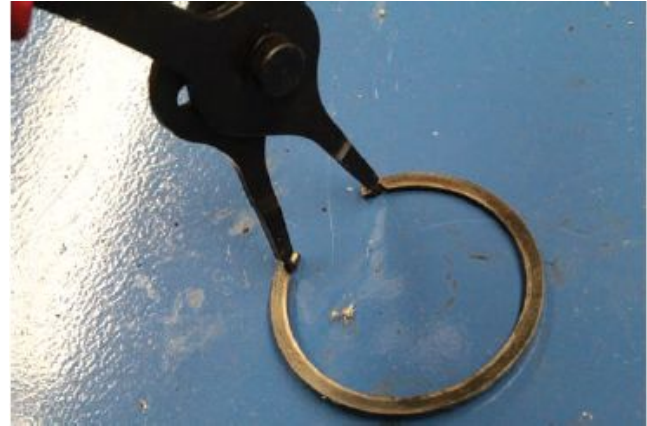
Snap ring pliers and snap ring.
