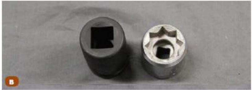
B. Four- and 8-point sockets.
