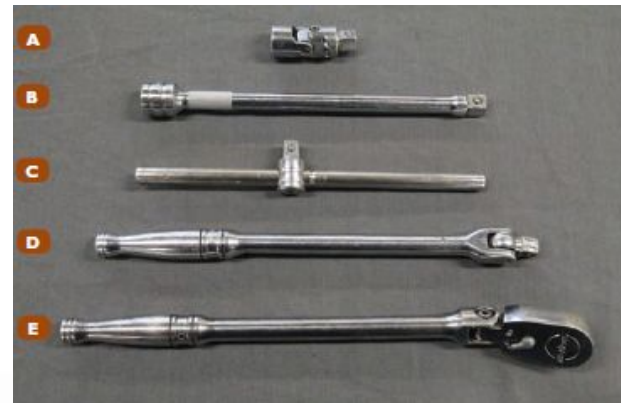
Tools to turn sockets. A. Universal joint. B. Extension. C. T-handle. D. Breaker bar. E. Ratchet.
