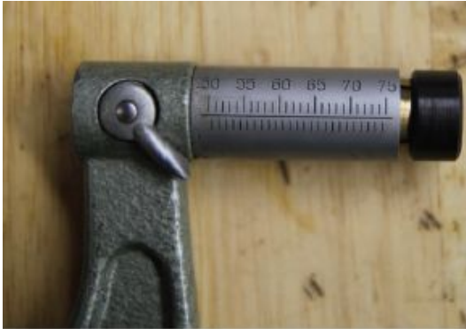
Metric markings on the sleeve.
