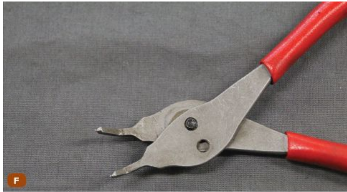
F. Internal snap ring pliers.
