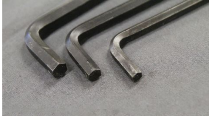
Typical Allen wrench head.
