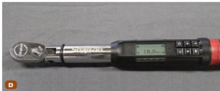
Torque wrenches. A. Beam style. B. Clicker style. C. Dial. D. Electronic.
