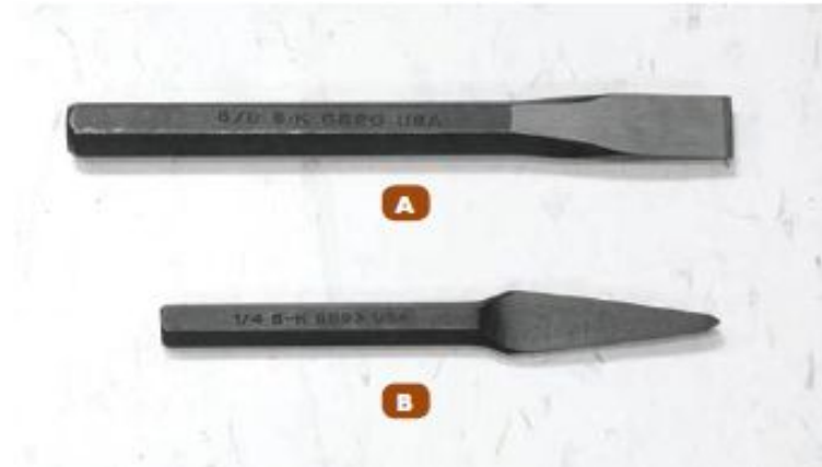
A. Cold chisel. B. Cross-cut chisel.
