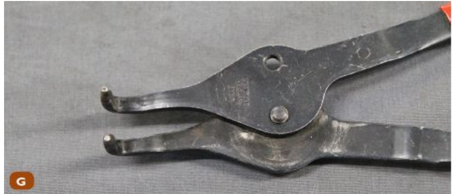
G. External snap ring pliers.
