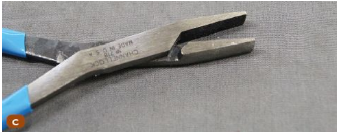
C. Flat-nose pliers.
