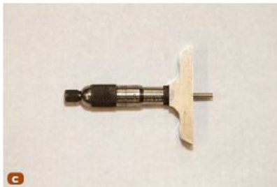
A. Outside micrometer. B. Inside micrometer. C. Depth micrometer.
