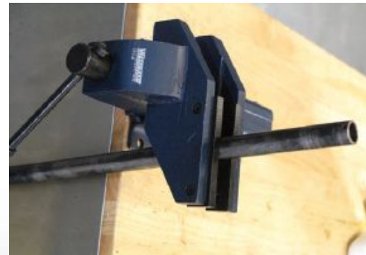
Offset vice being used to hold a pipe.
