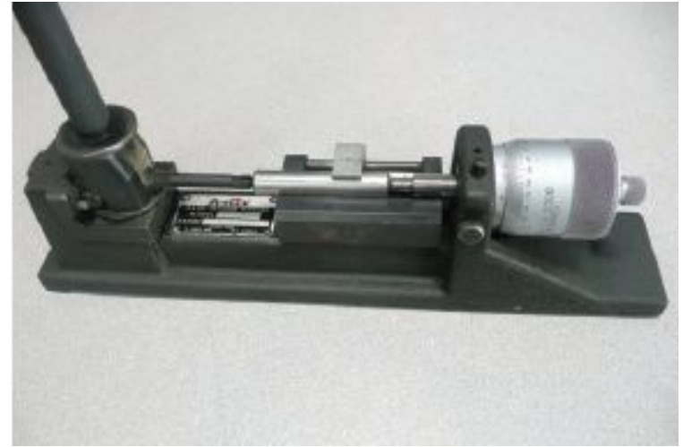
Dial bore gauge being calibrated to a predetermined size.
