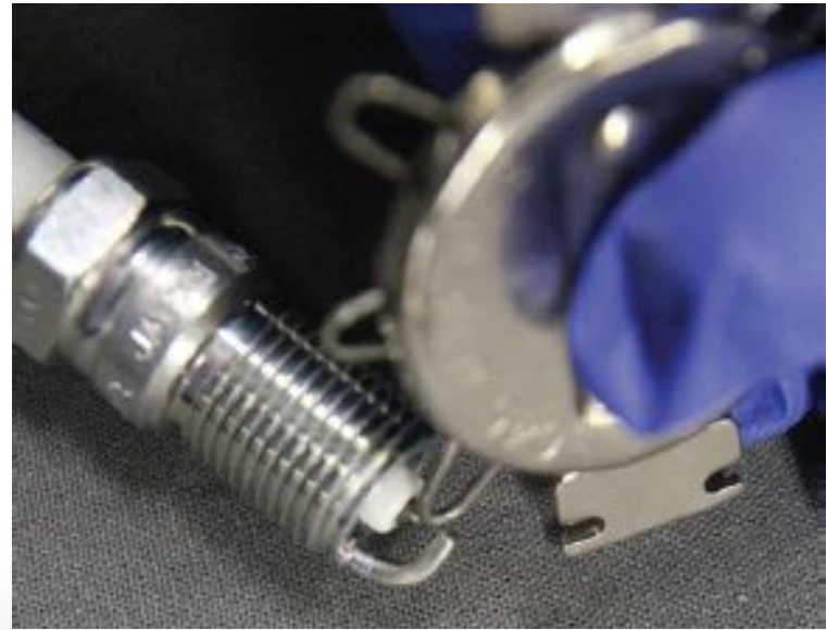
Wire feeler gauge used to check a spark plug gap.
