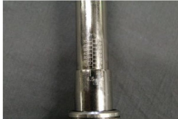
Torque setting scale on the handle.
