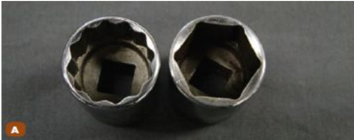
A. Six- and 12-point sockets.
