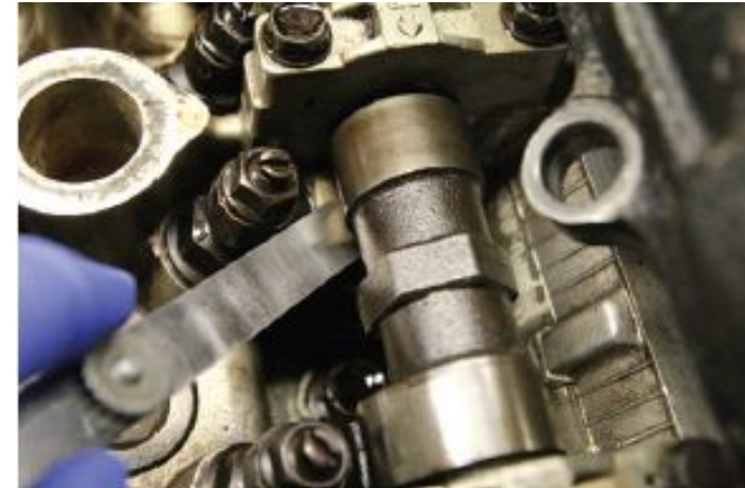
Stepped feeler blade being used during a valve adjustment.
