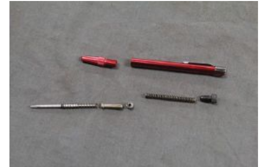
Internal workings of an automatic center punch.
