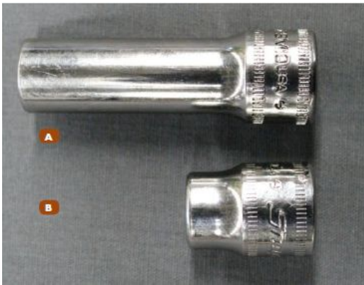
A. Deep socket. B. Standard length socket.
