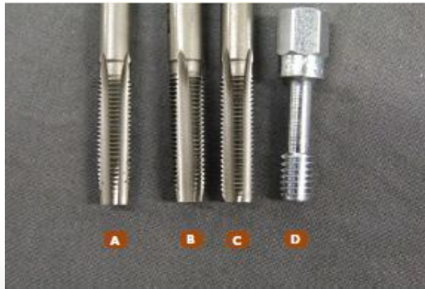
A. Taper tap. B. Intermediate tap. C. Bottoming tap. D. Thread chaser.
