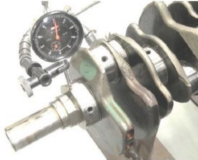
A dial indicator being used to measure crankshaft runout.
