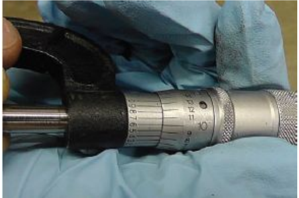
Vernier scale on a micrometer showing 7 on the sleeve lined up the best with a line on the thimble.
