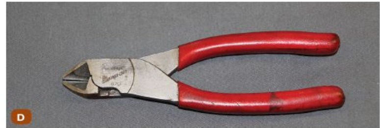
D. Diagonal cutting pliers.
