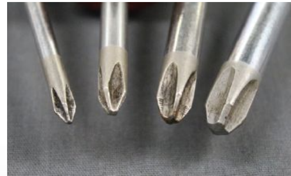
Four sizes of Phillips screwdrivers.
