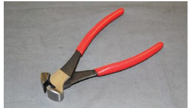
Nippers, or end cutting, pliers.
