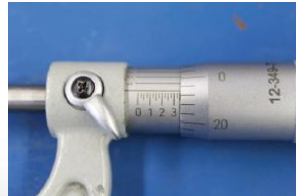
0.100" and 0.025" markings on the sleeve.
