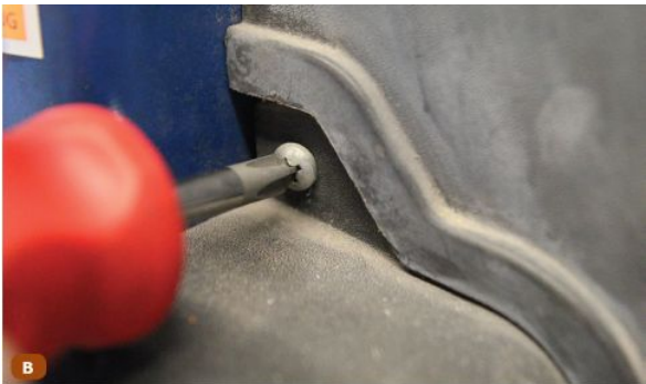
B. Phillips screw and screwdriver.
