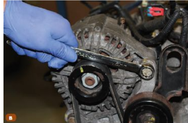
B. Pushing regularly results in bruised or broken knuckles.
