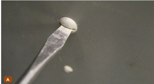
A. Slotted screw and screwdriver.
