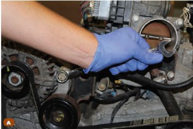
A. Pulling on a wrench is generally better than pushing on a wrench.
