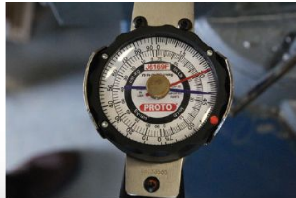
Dial torque wrench reading torque.
