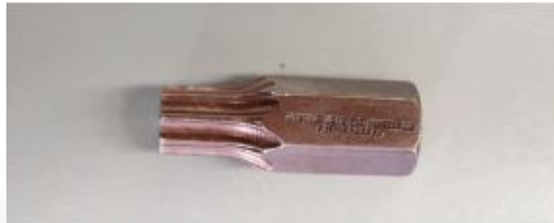
Straight-sided screw extractor.
